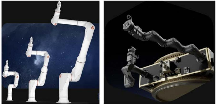
Fig. 26. Motive Space System's Robotic arms (left: xlink, right: modulin).
