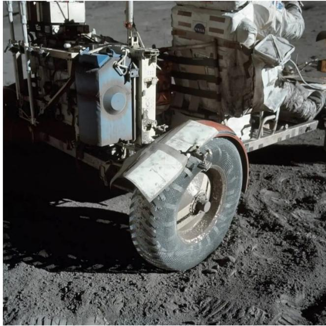
Fig. 4. Lunar dust contamination on the Apollo rover [64].
