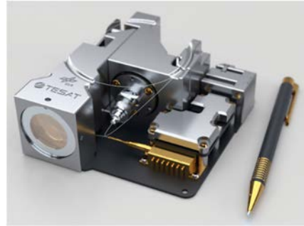
Commercial off-the-shelf laser communication terminal for cube satellite [Tesat-Spacecom]
