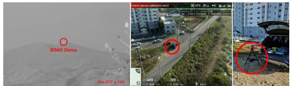
Fig. 10. Field of view of OCT at a distance of 20 km, including Bohyunsan Optical Astronomy Observatory (BOAO) (left). The received live streaming HDMI video at OGS (center) and the HDMI video transmitting OCT (right). OCT, optical communications terminal; HDMI, high-definition multimedia interface; OGS, optical ground station.
