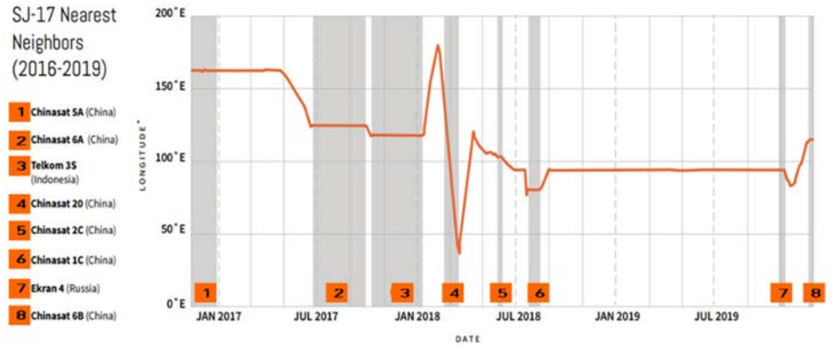
Fig. 7. RPO activities of China satellite against Indonesia satellite. RPO, Rendezvous and Proximity Operations.
