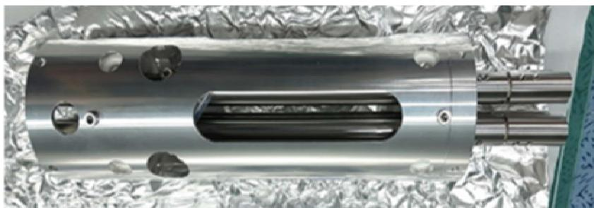
Fig. 9. Prototype quadrupole mass analyzer.
