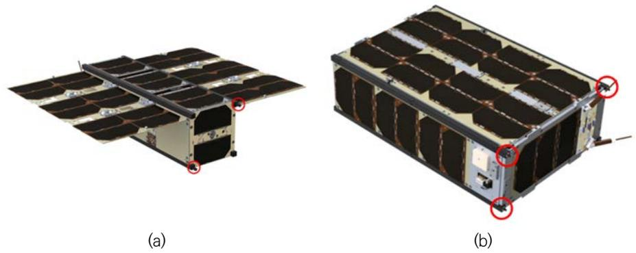
Fig. 2. Deployment switches of 3U(a) & 6U(b) of Gomspace.
