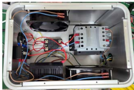
Fig. 4. Assembly of control part.
