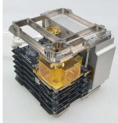
Fig. 4. SNiPE science payload. The SST, LP, and Mag are integrated into 1 unit.
