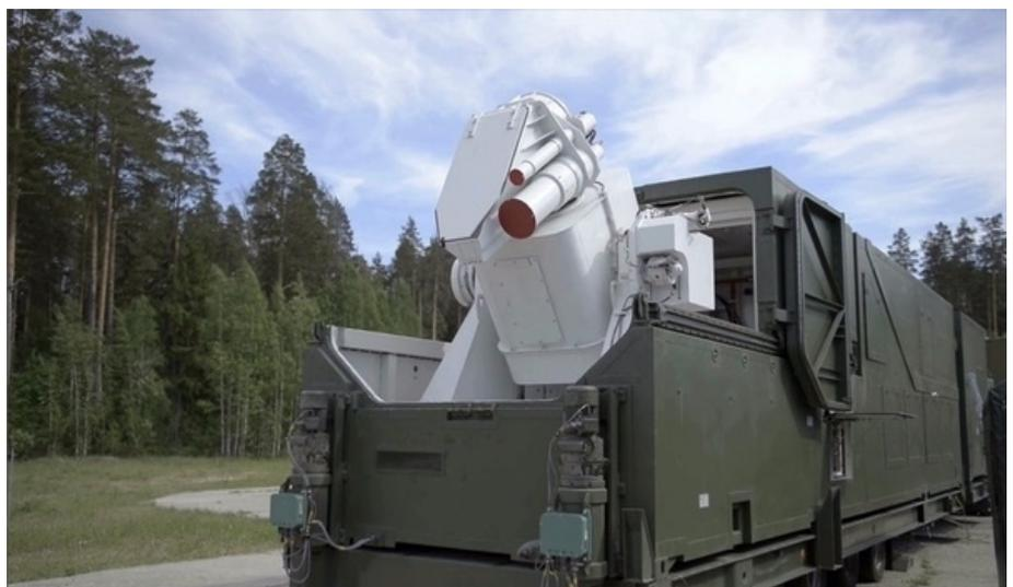
**Fig. 9.** Russia's Peresvet system, a publicly disclosed directed-energy ASAT weapon system [18]. ASAT, anti-satellite weapon.
