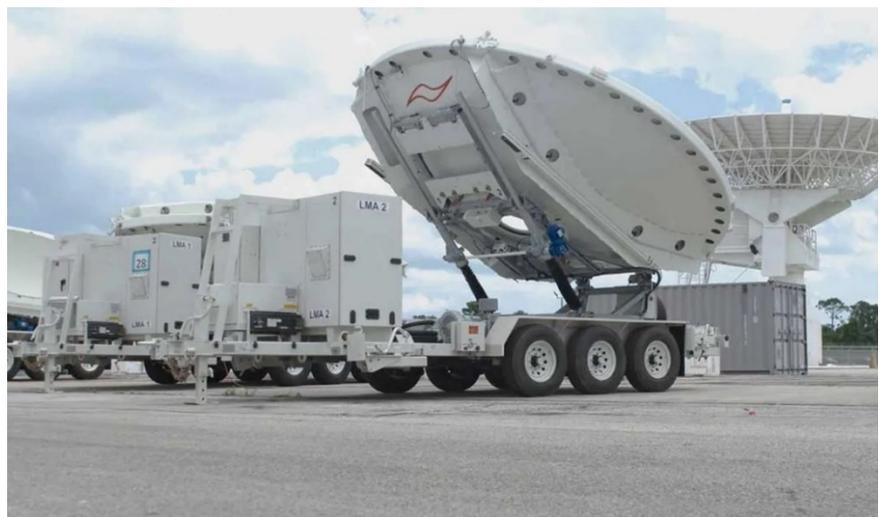
Fig. 6. The Meadowlands system: a satellite-based electronic warfare capability employed by the U.S. Space Force [10].
