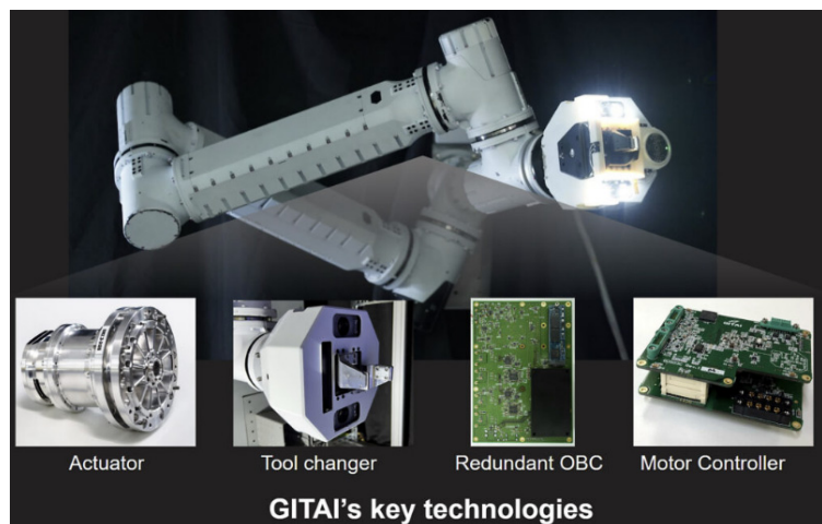
Fig. 24. GITAI Robotic Arm's key technologies.
