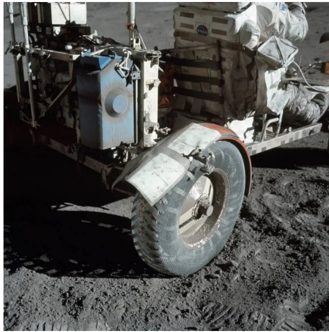
Fig. 4. Lunar dust contamination on the Apollo rover [64].
