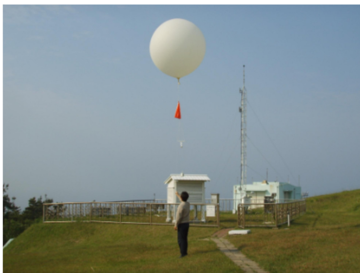
Fig. 2. Korea Meteorology Agency flying radiosonde using helium balloon [2].
