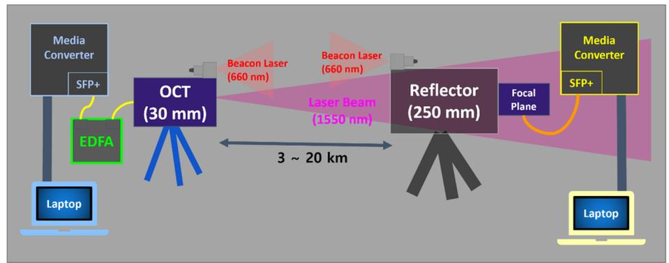
**Fig. 5.** Diagram of FSOC experiment with 4K HDMI live streaming system. OCT, optical communications terminal; EDFA, erbium-doped fiber amplifier; FSOC, free-space optical communication; HDMI, high-definition multimedia interface.
