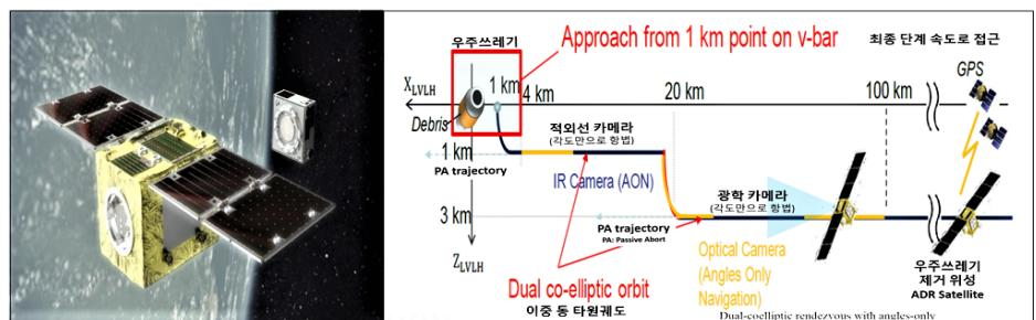
Fig. 12. Illustration of ELSA-d specific CONOPS of ADR. ELSA-d, end-of-life service by astroscale; ADR, active debris removal.
