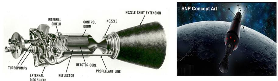
Fig. 25. Nuclear thermal propulsion engine & Chinese SNTP concept. SNTP, space nuclear thermal propulsion.
