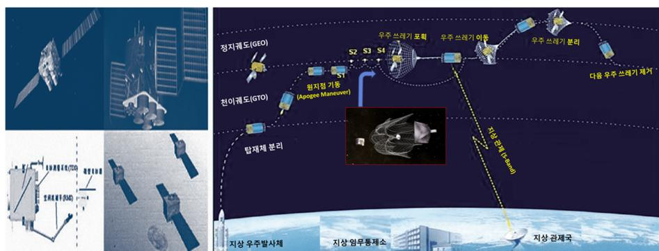
Fig. 9. ROBOTIC ARM DEMONSTRATOR SY-7 & ESA ADR Project CONOPS using Space Net. ESA, European Space Agency; ADR, active debris removal.
