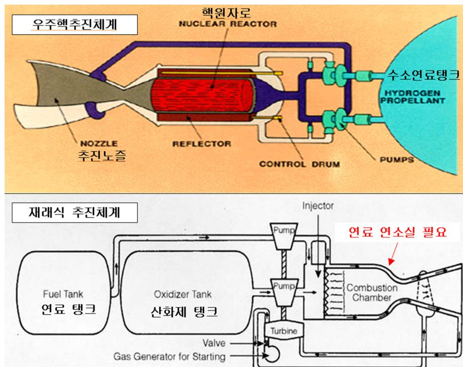
Fig. 31. Nulcear engine & chemical engine concept.
