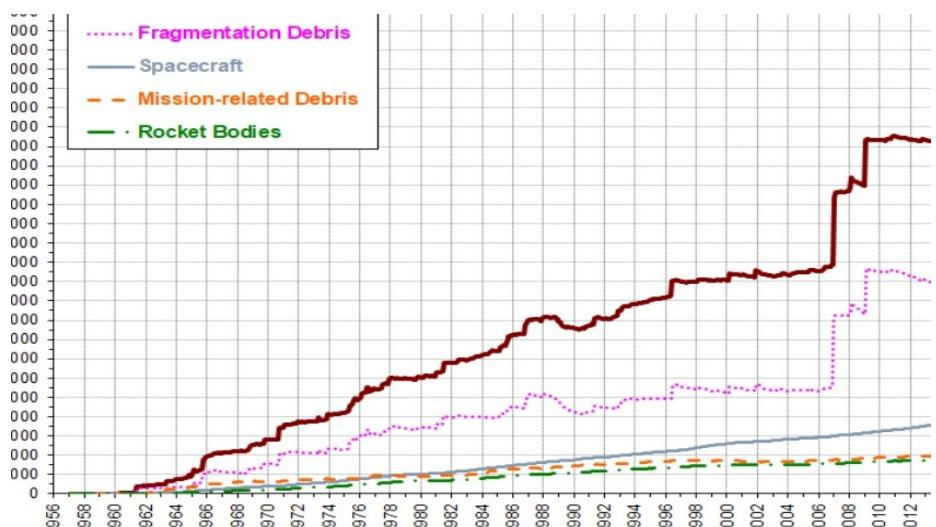
Fig. 2. Monthly number of objects in earth orbit by object type [6].
