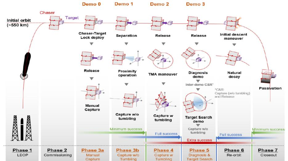
Fig. 11. Illustration of ELSA-d CONOPS. ELSA-d, end-of-life service by astroscale.
