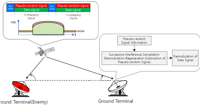
Fig. 7. Concept of physical layer security in downlink.
