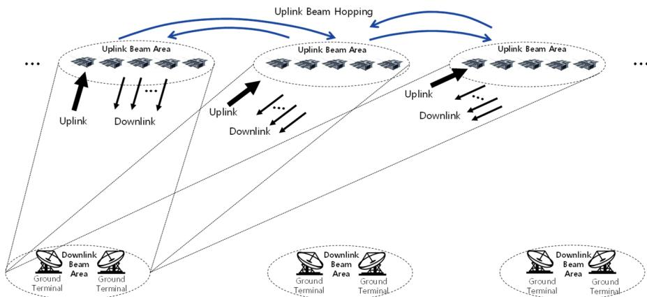
**Fig. 10.** Operation concept of future nanosatellite communication system.
