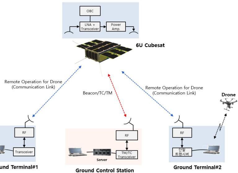
**Fig. 1.** Operation concept of the nanosatellite communication system. OBC, on-board computer; LNA, low noise amplifier; TC, telecommand; TM, telemetry; RF, radio frequency.
