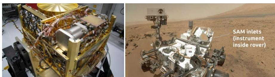
Fig. 6. Sample analysis at Mars (SAM) in Mars science laboratory (MSL) (Image credit: NASA).
