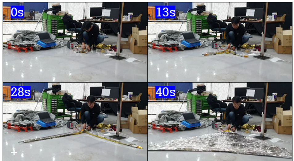
Fig. 11. Deployment test of 3 m sized drag device by active method.
